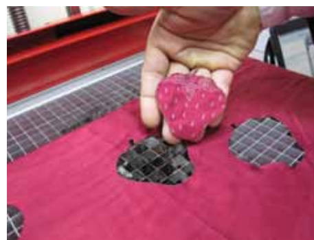
With optional software, a standalone laser can be programmed to do multiple jobs at once. Operators can use a double-sided tray and move back and forth between two or more jobs with the click of a button.
