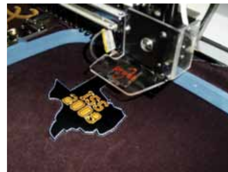
The most affordable option for small to mid-size shops for cutting emblems is the single-head embroidery laser, which speeds up production by sewing the emblem, and then the needle bar, which has the laser attached to it, comes back and cuts it out.
