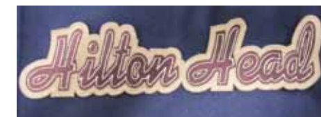
One advantage of using a laser to cut patches is it opens the door to a greater variety of fabrics than is available using traditional methods. This Hilton Head patch, created by Pittsburgh-based Stitches, features felt on top of athletic twill.
